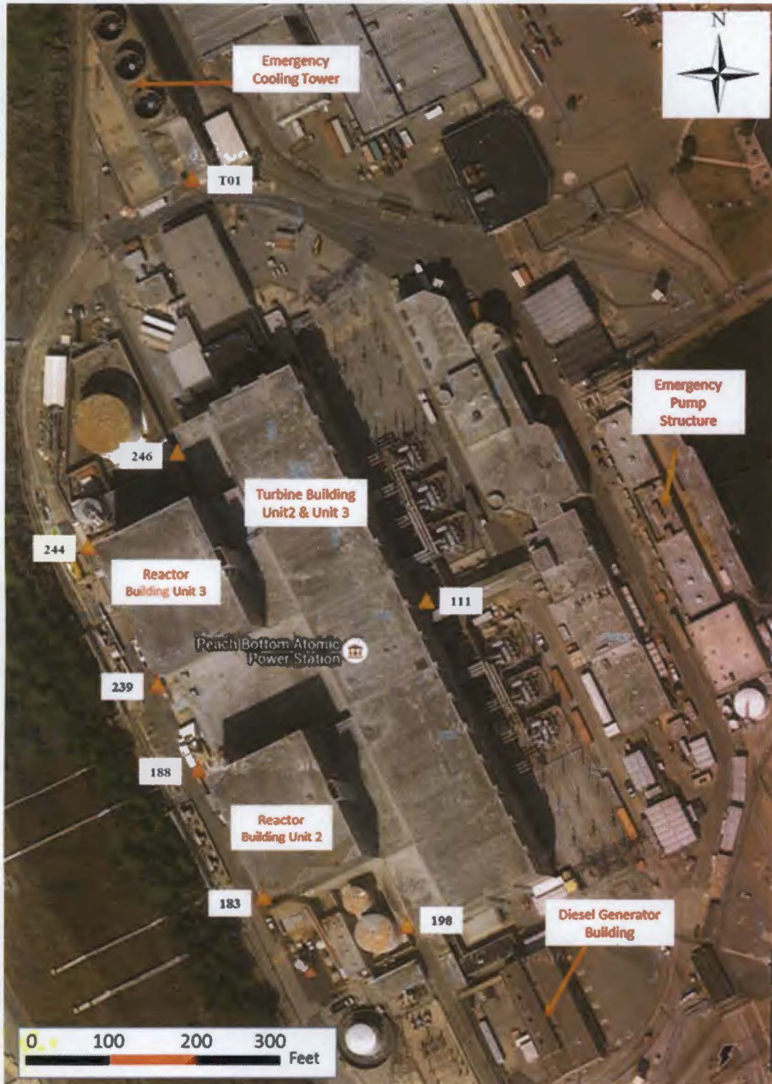
Figure 3.2-1. Location map showing the critical locations, which were evaluated in the LIP analysis, including (1) seven doors of safety-related structures, (2) one door of Turbine Building, which is not a safety-related structure, and (3) two other critical structures (Diesel Generator and Pump Structure) that are associated with five evaluated critical locations.
