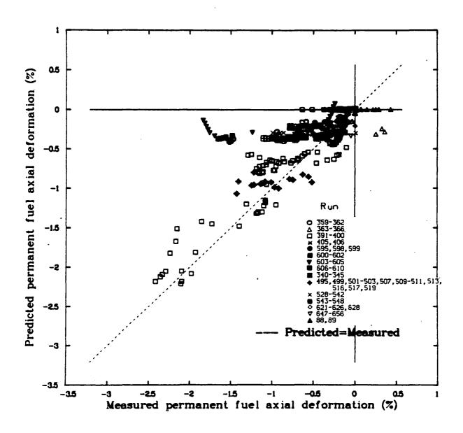
Fig. 7 FRAPCON-1 predicted against measured permanent fuel axial deformation.
