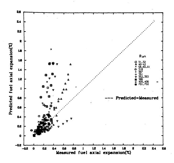
Fig. 6 FRAPCON-1 predicted against measured fuel axial expansion during heatup.
