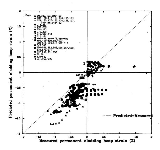
Fig.  $\ensuremath{\mathfrak{B}}$  FRAPCON-1 predicted against measured permanent cladding hoop strain.
