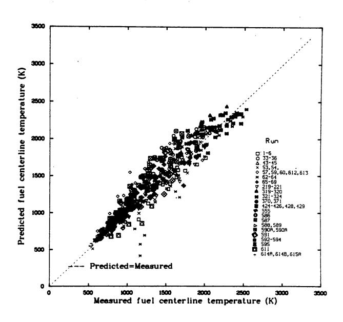
Fig  $\P$  FRAPCON-1 predicted against measured centerline temperatures for unpressurized rods.
