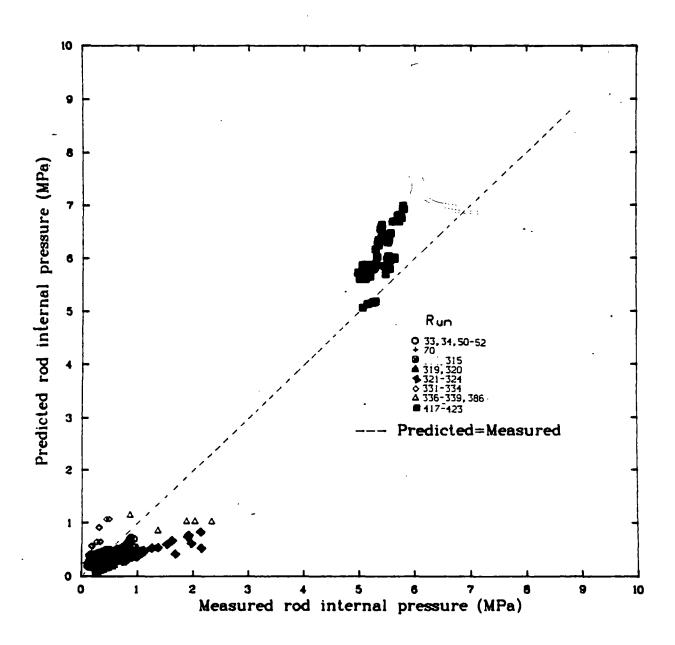
Fig. 5 FRAPCON-1 predicted against measured rod internal pressure at high burnup conditions.
