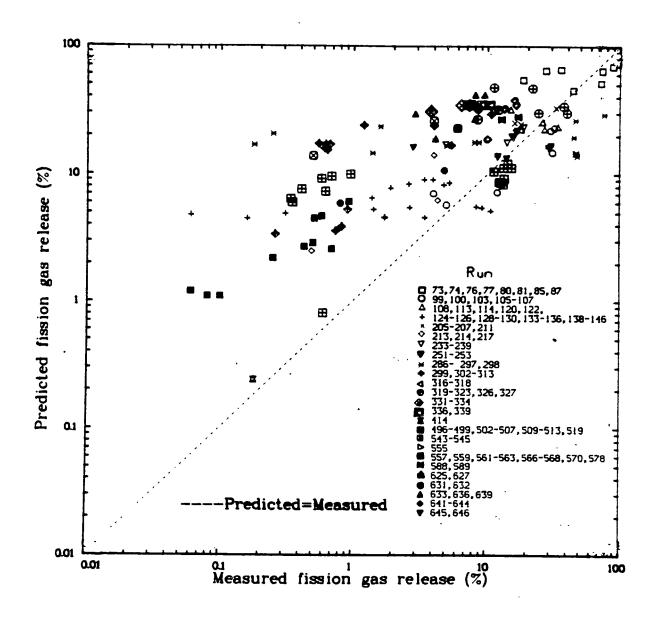
Fig.  $\bf 3$  FRAPCON-1 predicted against measured fission gas release fraction.
