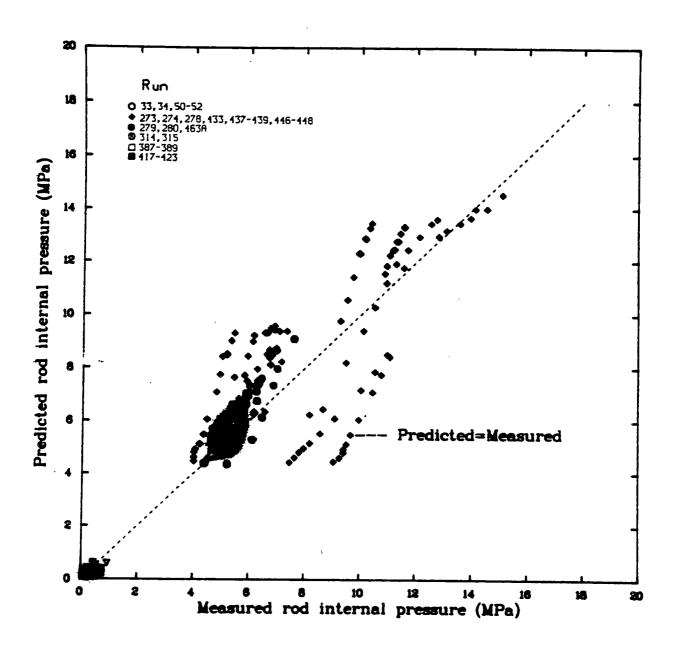
Fig. 4 FRAP CON-1 predicted against measured rod internal pressure
