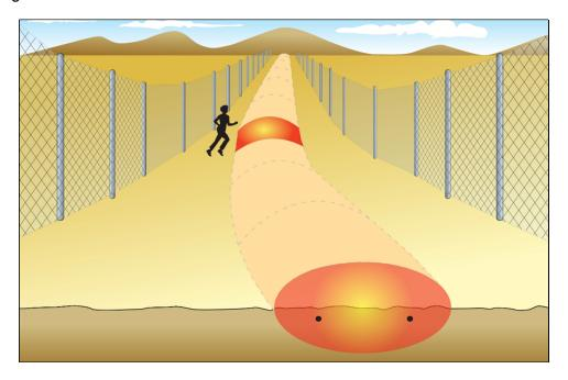
Figure 16 An illustration of the covert zone of detection for a ported coaxial sensor
