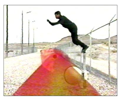
Figure 6 Microwave mounting structure used to jump over the detection zone
