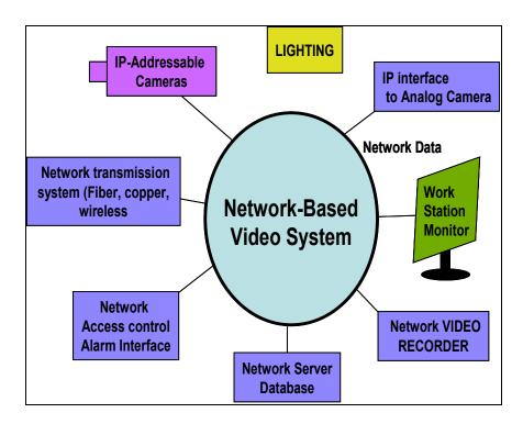
Figure 60 Diagram of a network-based digital video system
