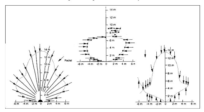
Figure 42 Differences in detection patterns from microwave sensor walk tests
