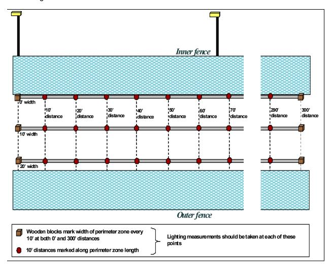
Figure 78 Points at which light readings should be measured
