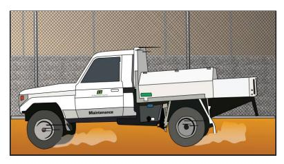
Figure 19 Example of a nuisance alarm source for ported coaxial cable detection systems
