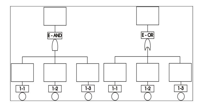
Figure 82 Fault trees used to analyze system events
