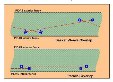
Figure 25 Active infrared sector intersection method
