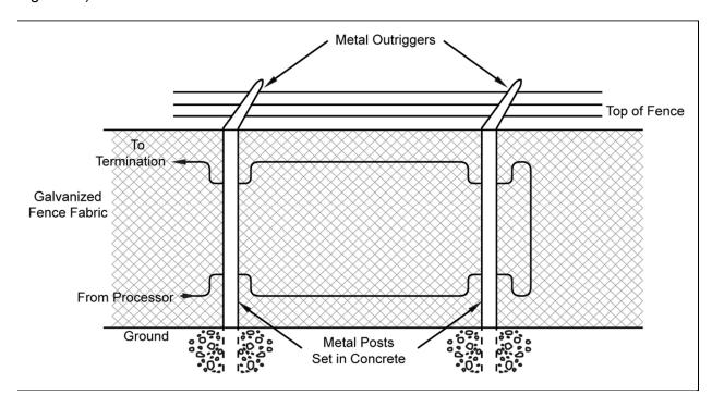
Figure 32 Typical installation of strain-sensitive cable
