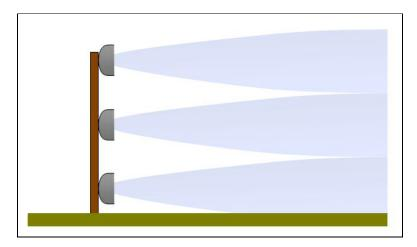
Figure 7 An example of stacked microwave sensors
