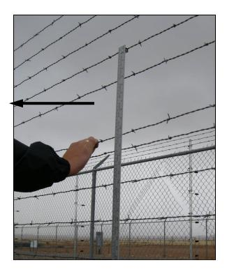
Figure 30 Measuring deflection on a taut wire sensor
