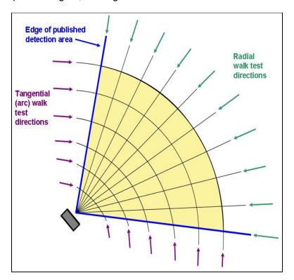
Figure 43 Recommended walk test paths for microwave sensor performance testing
