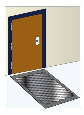
Figure 54 Example of a mat sensor near a door
