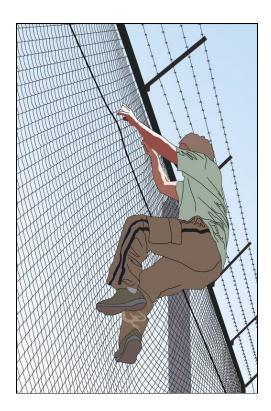
Figure 31 Deflection caused by an intruder climbing on chain-link fence fabric
