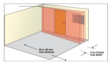
Figure 46 An example of a curtain PIR application
