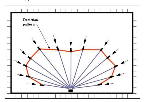
Figure 49 A typical PIR detection pattern derived from walk tests toward the sensor
