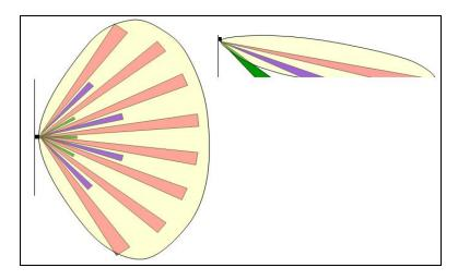
Figure 55 Example of a dual-technology sensor
