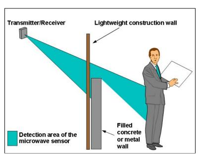
Figure 41 A microwave sensor triggering a nuisance alarm
