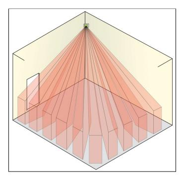
Figure 45 Example of a PIR sensor's subdivided detection pattern
