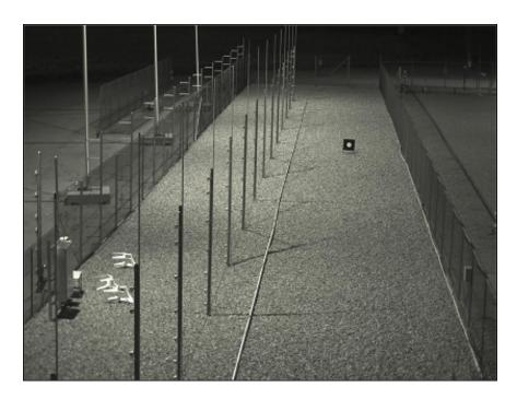
Figure 70 Improved assessment visibility with even lighting and a regular ground surface
