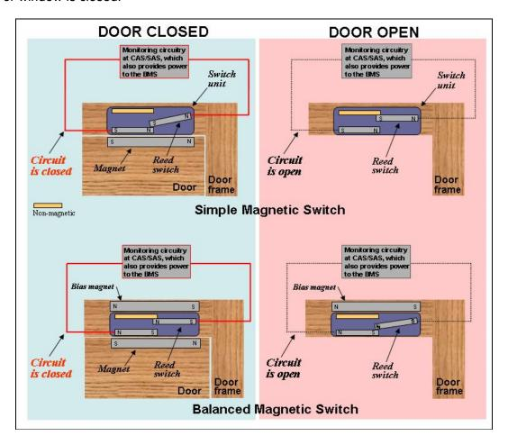
Figure 37 A schematic of a simple switch versus a BMS
