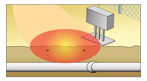
Figure 21 Example of metal objects or utilities located near a ported coaxial system
