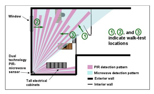
Figure 56 Walk test areas in a room covered by a dual-technology PIR-microwave sensor
