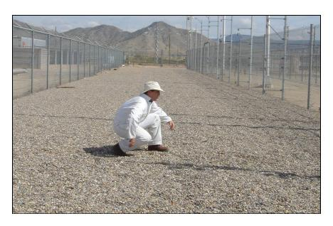
Figure 22 The duck walk test method for a ported coaxial system
