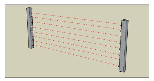
Figure 23 Multibeam active infrared sensor columns
