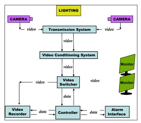
Figure 59 Diagram of an analog video system
