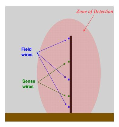
Figure 11 A cross-section of an electric field sensor's zone of detection
