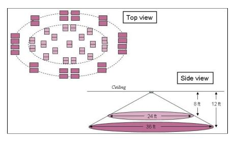
Figure 47 Illustration of the detection pattern of a ceiling-mounted PIR
