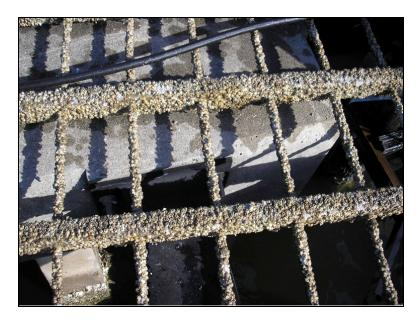
Figure 58 Example of degradation of underwater fiber-optic grid sensors
