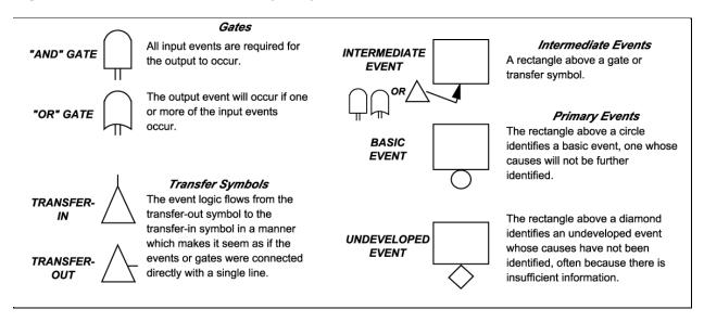
Figure 83 Symbols used in the graphical representation of a fault tree
