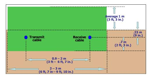
Figure 17 A typical installation and detection envelope (green) for a ported coaxial sensor
