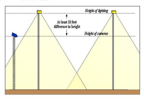
Figure 74 Recommended height differences between exterior lighting and cameras
