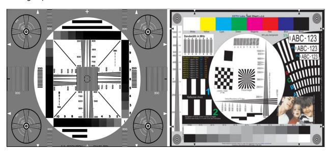
Figure 61 Examples of laboratory black and white and color camera resolution charts (graphic courtesy of CCTV Labs, available at www.cctvlabs.com)
