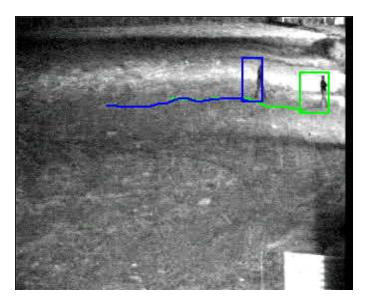
Figure 68 VMD image showing intruder tracking
