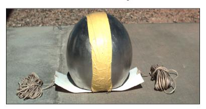
Figure 8 Aluminum sphere used to simulate crawl tests of the microwave detection system
