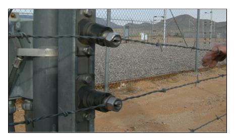
Figure 28 Taut wire push test
