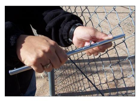
Figure 34 Use of a fence-cut simulation tool
