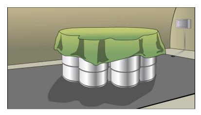
Figure 52 Example of a pressure mat
