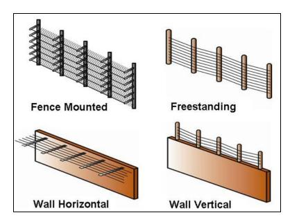
Figure 12 Various configurations for electric field sensors
