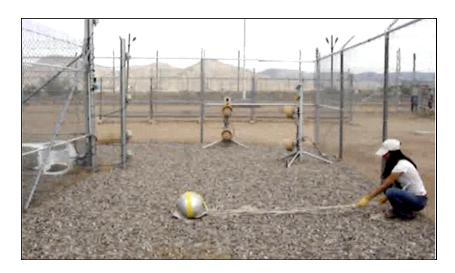
Figure 9 Testing of microwave sensors with an aluminum sphere
