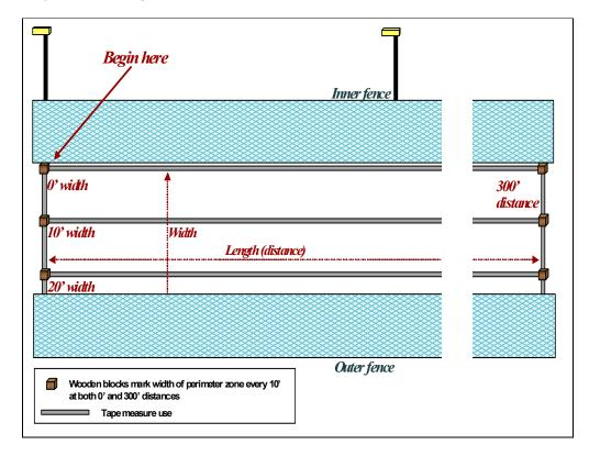
Figure 77 Preparation for measuring perimeter lighting illumination
