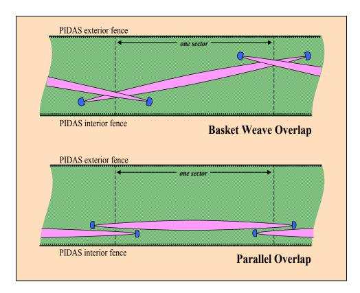
Figure 4 Examples of possible microwave sensor layouts
