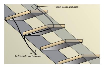
Figure 53 Strain sensor concept to detect an intruder on stairs
