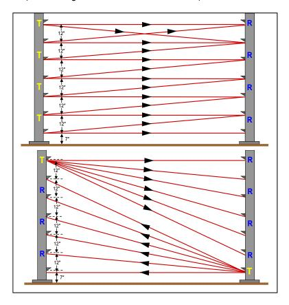
Figure 24 Active infrared sensor variations in beam configuration
