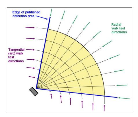
Figure 48 Recommended walk tests for the performance testing of a PIR sensor
