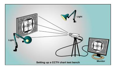
Figure 62 Example of a resolution chart test setup
