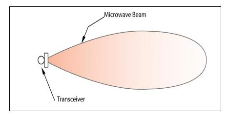
Figure 39 A common interior microwave antenna propagation pattern
