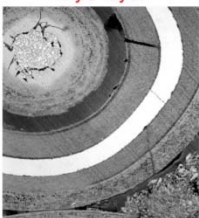
Particle with cracked IPyC layer
