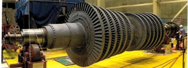
High Pressure Turbine
