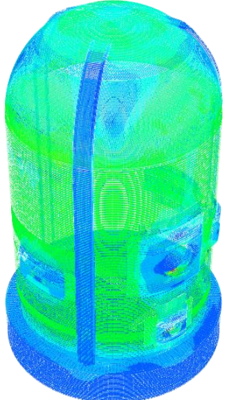
Strain contour of tendon, rebar, and liner plate
