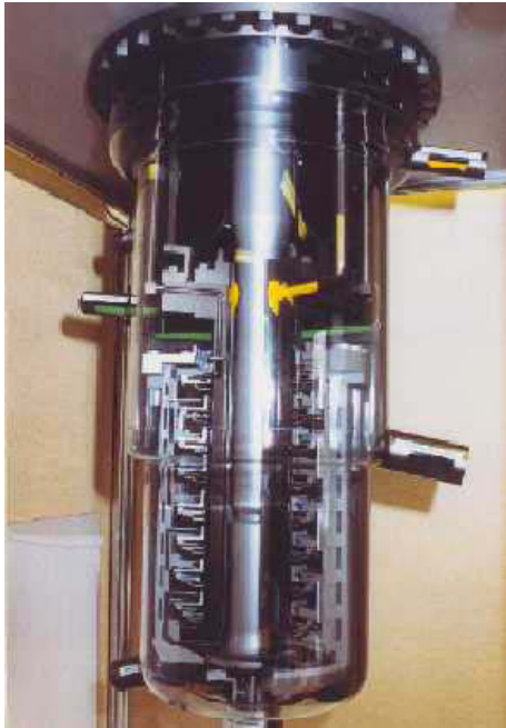
Figure B-28 Cut away view of a multi-stage centrifugal contactor [Drain 2003]
