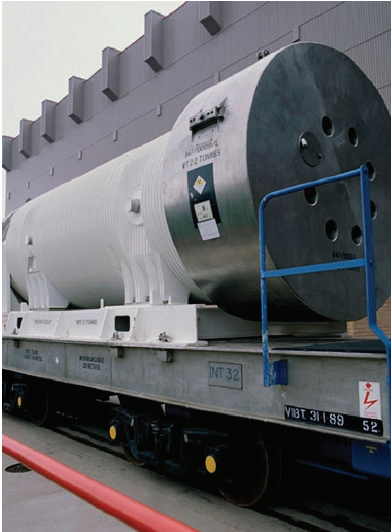
Spent fuel cask on rail transport.
