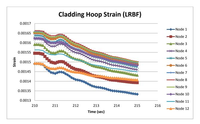
Figure 39 Cladding hoop strain of LRBF transient
