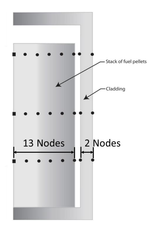
Figure 3 Setting of radial nodes in FRAPTRAN model
