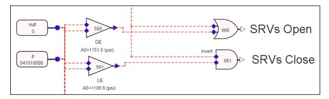
Figure 13 Controlling system of relief valves in TTBF hypothetical accident
