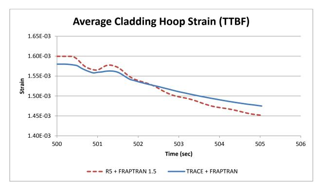
Figure 32 Cladding hoop strain comparison of TTBF transient
