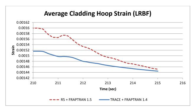
Figure 42 Cladding hoop strain comparison of LRBF transient
