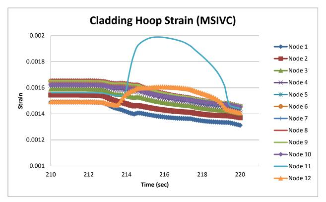
Figure 20 Cladding hoop strain of MSIVC transient
