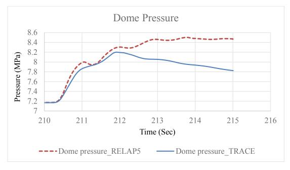
Figure 35 Dome pressure variation during the LRBF hypothetical accident
