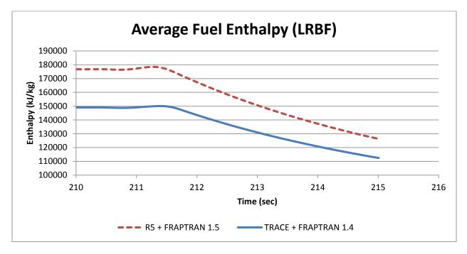
Figure 43 Fuel enthalpy comparison of LRBF transient
