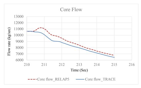
Figure 37 Core flow variation during the LRBF hypothetical accident
