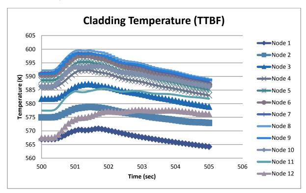
Figure 28 Cladding temperature of TTBF transient
