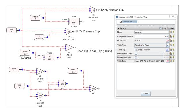
Figure 12 Controlling system of reactor scram in TTBF hypothetical accident
