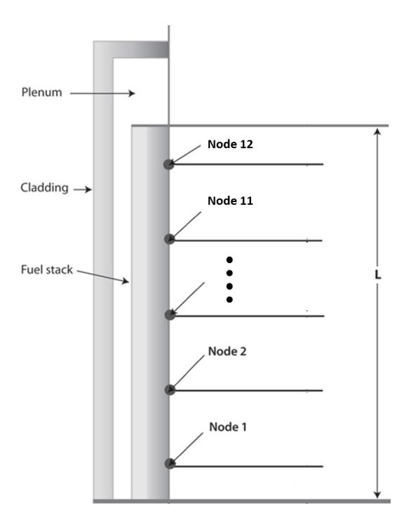
Figure 4 Setting of axial nodes in FRAPTRAN model
