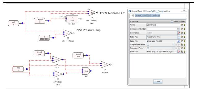
Figure 10 Controlling system of reactor scram in MSIVC hypothetical accident
