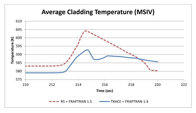
Figure 22 Cladding temperature comparison of MSIVC transient
