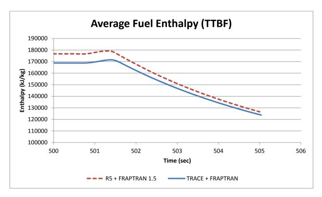
Figure 33 Fuel enthalpy comparison of TTBF transient
