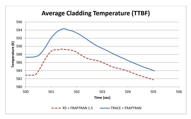
Figure 31 Cladding temperature comparison of TTBF transient
