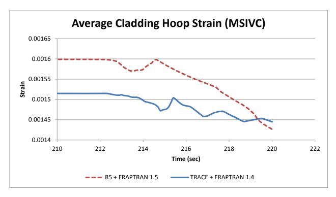
Figure 23 Cladding hoop strain comparison of MSIVC transient
