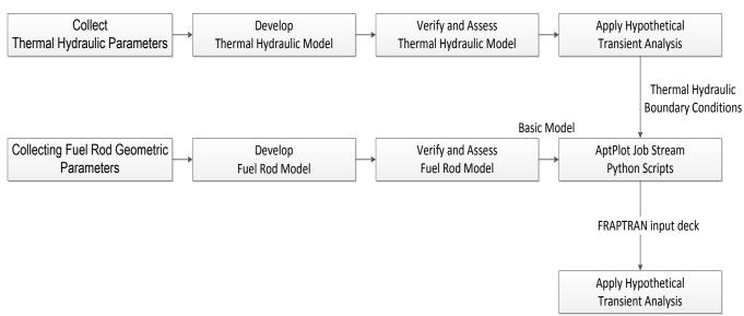
Figure 1 Flow chart of thermal hydraulic and fuel rod mechanism analysis model
