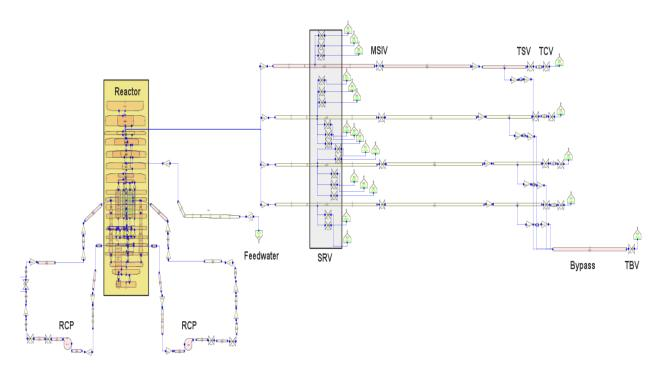
Figure 2 Overview of the Kuosheng NPP RELAP5/MOD3.3 model
