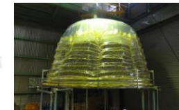
Sealing a PCV head (1:4 scale) with Radioactive material diffusion preventing film
