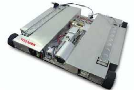
313mm(L) × 327mm(W) × 47mm(H) (Toshiba)
