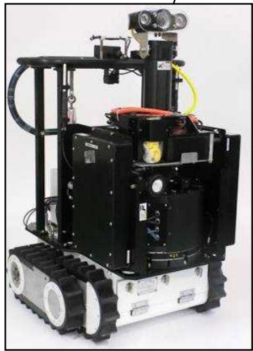
Investigation device for the upper part of the S/C (IRID)
