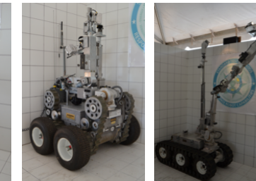
Remotec Mark 5-A 358kg (790lbs) Remotec Wolverine 367kg (810lbs)
