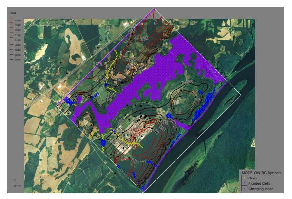
Figure 40. Hydraulic head contours (every 2 feet) resulting from the initial PEST calibration
