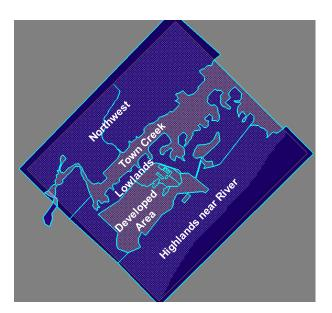
Figure 53. Refined recharge zones for the post-construction scenario. A portion of the Lowlands zone was incorporated into the northern corner of the Developed Area zone.
