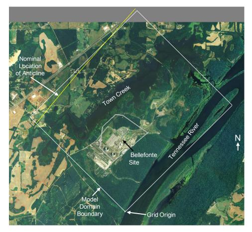
Figure 22. Extent of the groundwater simulation model grid relative to key features. The grid origin is located in the lower left corner of the model at the bottom of the domain.
