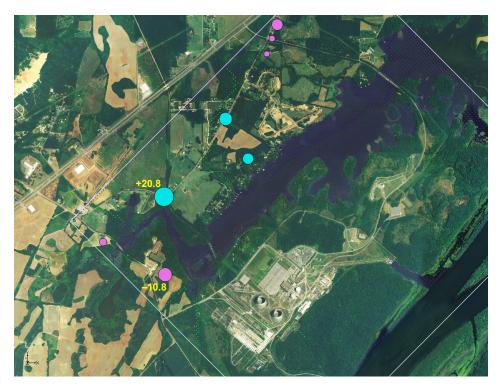
Figure 41. Unweighted residuals (observed minus simulated, in feet) for the 1961 data. Positive (blue) and negative (pink) residual magnitudes are proportional to symbol size.
