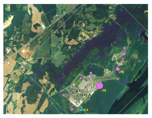
Figure 42. Unweighted residuals (observed minus simulated, in feet) for the September 2005 data. Positive (blue) and negative (pink) residual magnitudes are proportional to symbol size.
