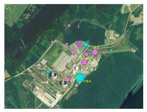
Figure 43. Unweighted residuals (observed minus simulated, in feet) for the average 2006/2007 "Bedrock" data. Positive (blue) and negative (pink) residual magnitudes are proportional to symbol size.
