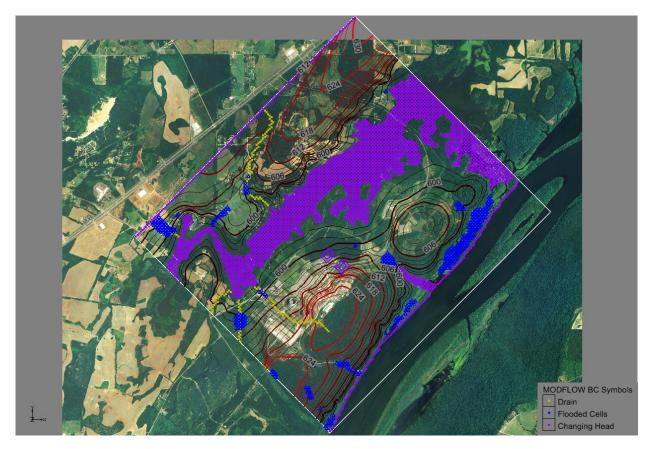
Figure 56. Hydraulic head contours for model H4R1D1 with the post-construction model configuration modifications. The purple rectangles indicate the location of Units 3 and 4, where inactive cells represent building foundations and fill material surrounds the foundations.
