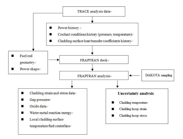
Figure 1 The Flowchart of Combining TRACE /FRAPTRAN/DAKOTA Codes
