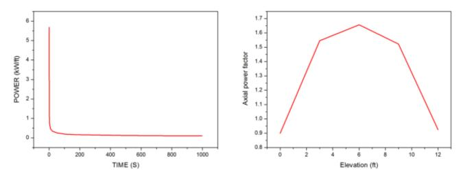
Figure 11 The Power History after Scram from TRACE (Left) and the Axial Power Shape of the Fuel Rod (Right)
