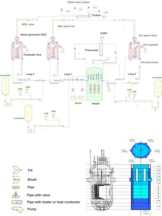
Figure 2 The LBLOCA TRACE Model of Maanshan NPP
