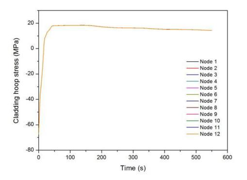
Figure 15 The Hoop Stress Variations during Transient at T03 Zone
