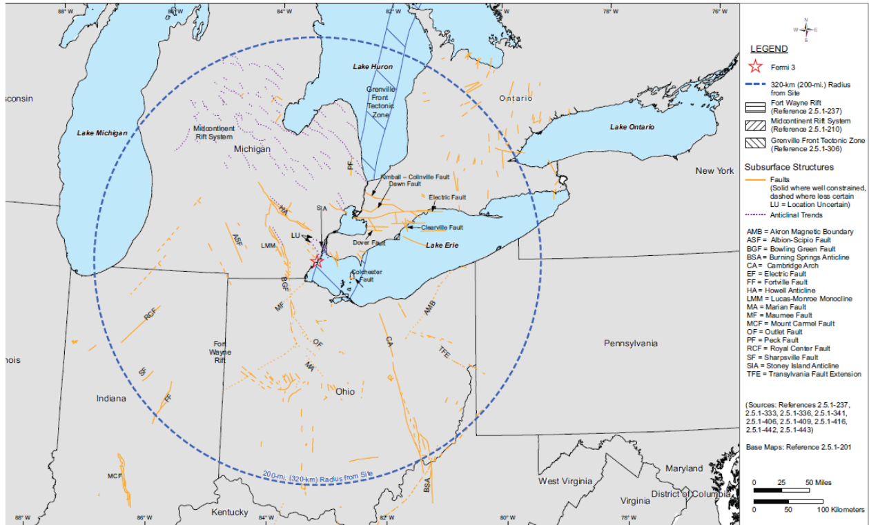
Figure 2.5.1-3 Fermi 3 Site Region Map of Tectonic Structures (Reproduced from Fermi 3 COL FSAR Figure 2.5.1-203)
