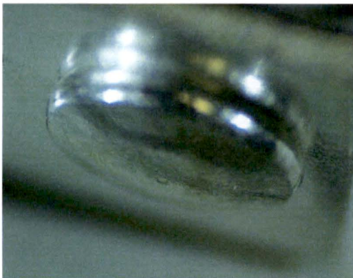
Figure 13: Contact rivet pre-aging
