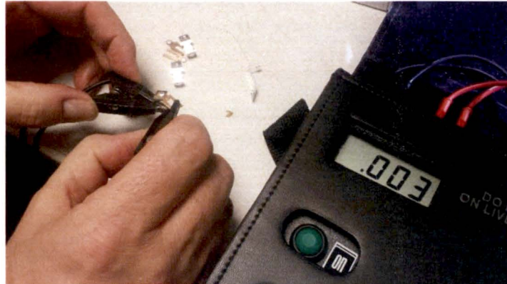
Figure 12: Resistance checks of contacts removed from switches
