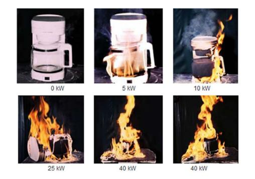
Figure 2-1 Fire Size/Intensity Calibration (0 to 40 kW)
