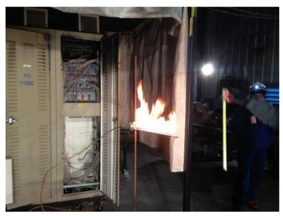
Figure 4-4. Photograph of 30 cm (12 in) propane line burner.
