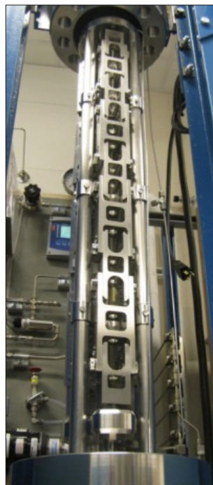
Figure 11.8 PWSCC initiation testing rig and 1.2-inch-tall specimen developed by PNNL.
