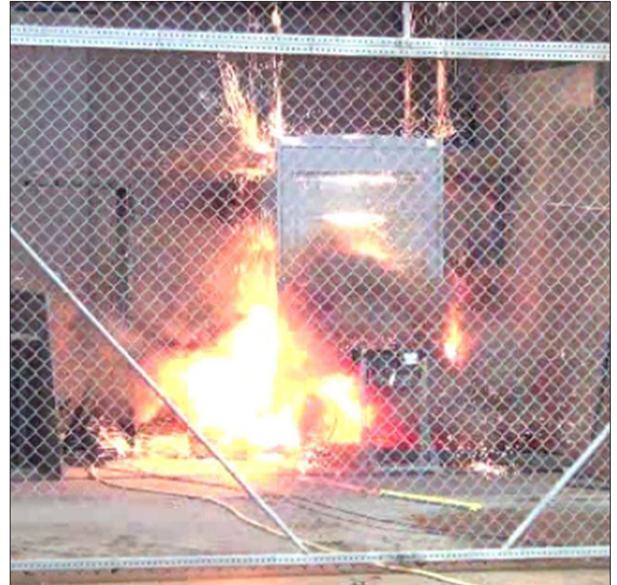
Figure 9.2 High Energy Arc Fault Testing of Electrical Components.
