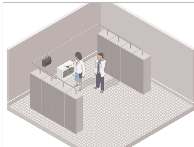
Figure 9.10 Illustration of operator response to aspirated smoke detection within an electrical enclosure.
