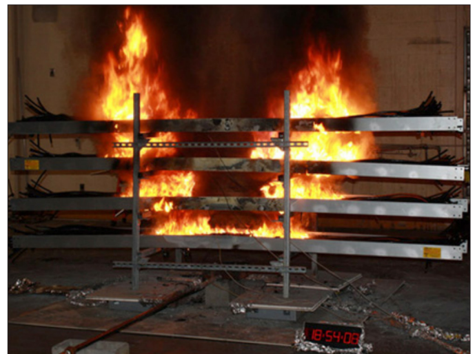
Figure 9.6 Burning cables during cable tray fire test (side view of burning cables in trays during a multiple-tray test after ignition using a small gas burner).
