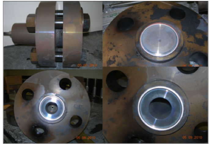
Figure 9.7 Pictures of the small-scale test vessel after 800 degrees C exposure for 9 hours (small-scale test vessel [top left], vessel head after disassembly [top right], and vessel body and metallic seal after disassembly [bottom left and bottom right]).
