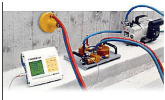
Figure 1.3 In-site surface air concrete permeability test apparatus.
