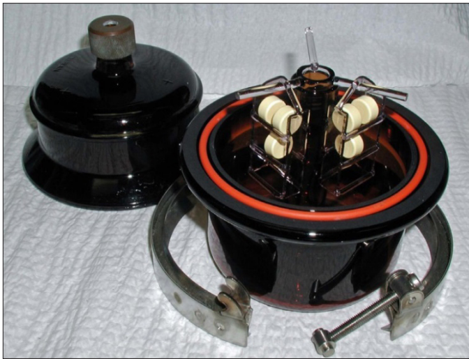
Figure 4.11 BIP irradiation vessel with sample coupons.
