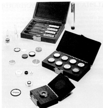
Figure 5-1. Calibration and Reference Sources. Calibration and reference sources may not need NRC or Agreement State registration.
