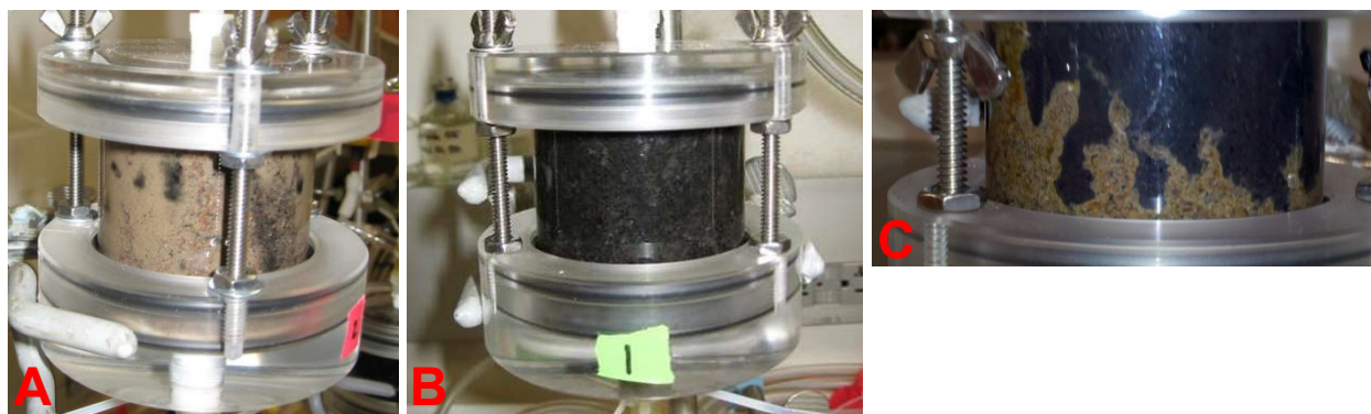
Figure 8. Column A 26 days after the start of biostimulation (A), at the end of biostimulation (B), and after oxic elution (C). Photographs by C. Fuller.
