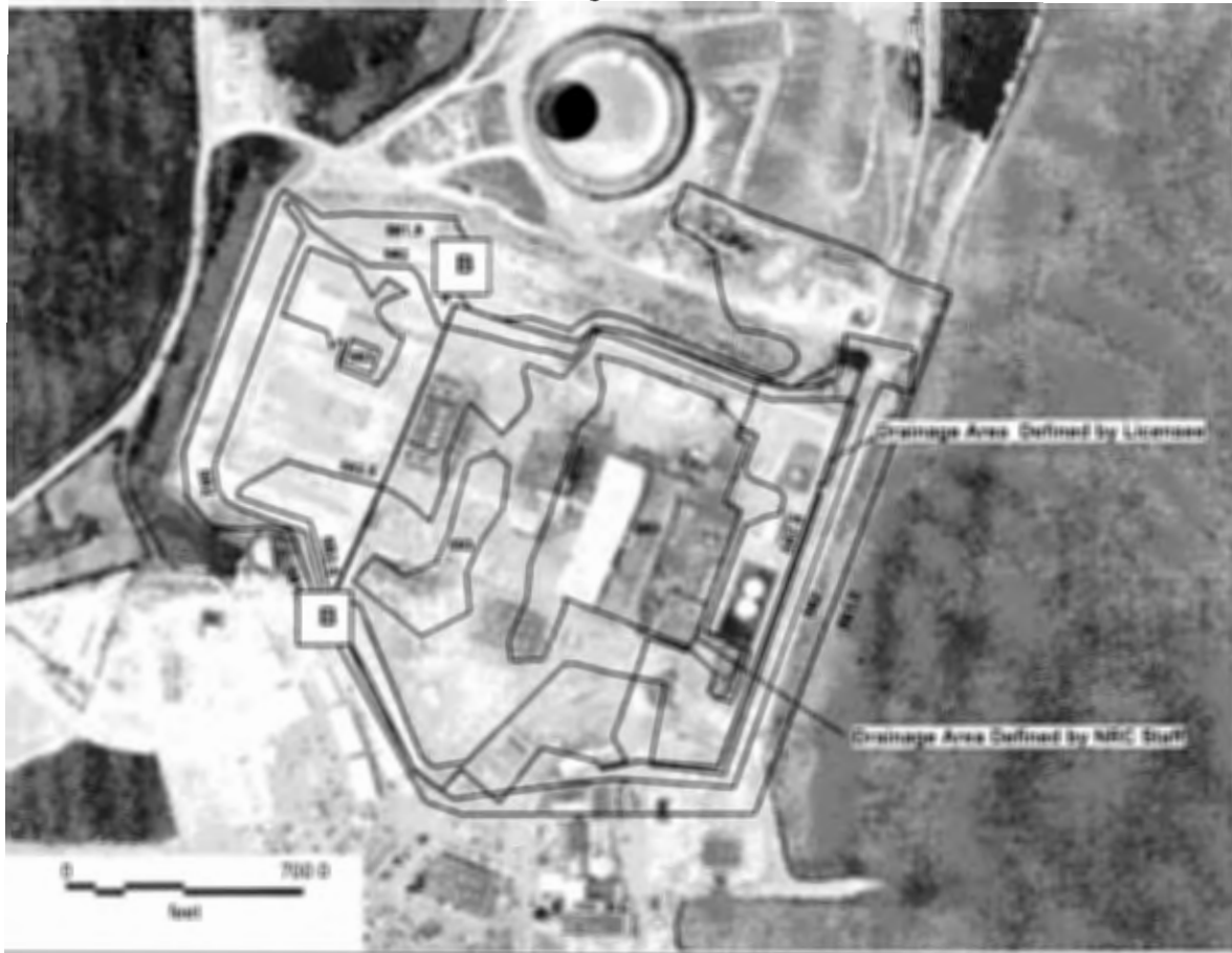
Figure 3.2-2: Site Map Showing Structures, Ground Surface Contour, Location of Cross Section B and Drainage Areas for Cross Section B.
