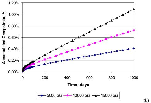
Figure 2.9 Cladding creep strain as a function of time and hoop stress for 630°F and flux=10<sup>18</sup> n/m<sup>2</sup>/s for (a) SRA Zircaloy and (b) RXA Zircaloy
