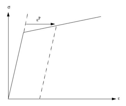
Figure 2.7 Typical isothermal stress-strain curve
