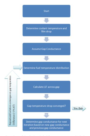
Figure 2.2 Flow chart of the fuel and cladding temperature calculation
