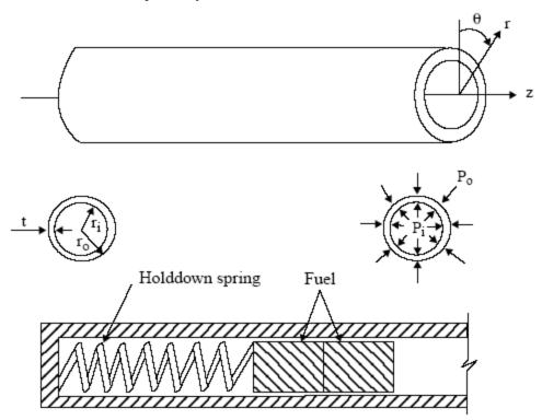
Figure 2.10 Fuel rod geometry and coordinates
