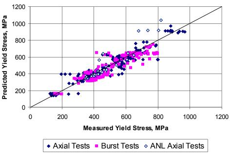
**Figure 2.14** Predicted vs. measured yield stress from the PNNL database  $(293K \le T \le 755K)$ ,  $0 \le \Phi \le 14x10^{25}$  n/m<sup>2</sup>,  $0 \le H_{ex} \le 850$  ppm
