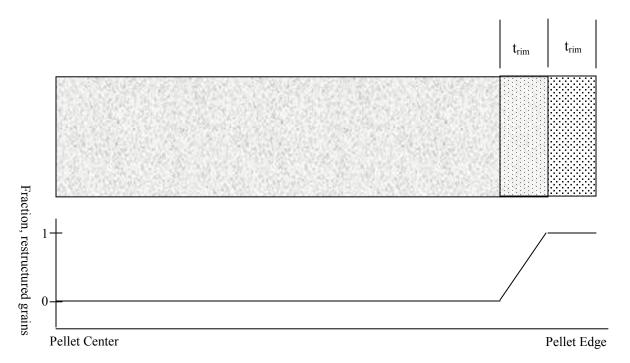
**Figure 2.17** Modeling the pellet high burnup rim structure in FRAPFGR
