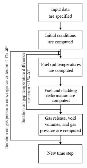
Figure 2.1 Simplified FRAPCON-3 flowchart
