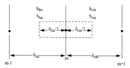
Figure 2.5 Typical mesh points
