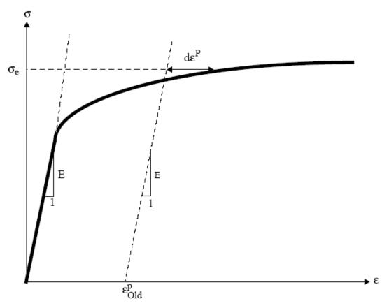
**Figure 2.11** Calculation of effective stress  $\sigma_e$  from  $d\epsilon^P$
