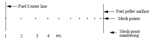
Figure 2.4 Mesh point layout
