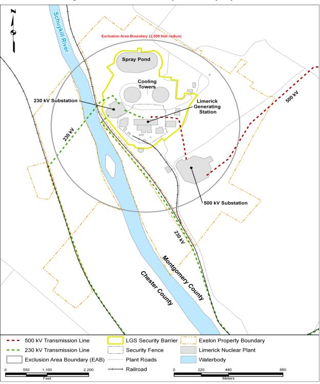
Figure 2–3. LGS Site Boundary and Facility Layout
