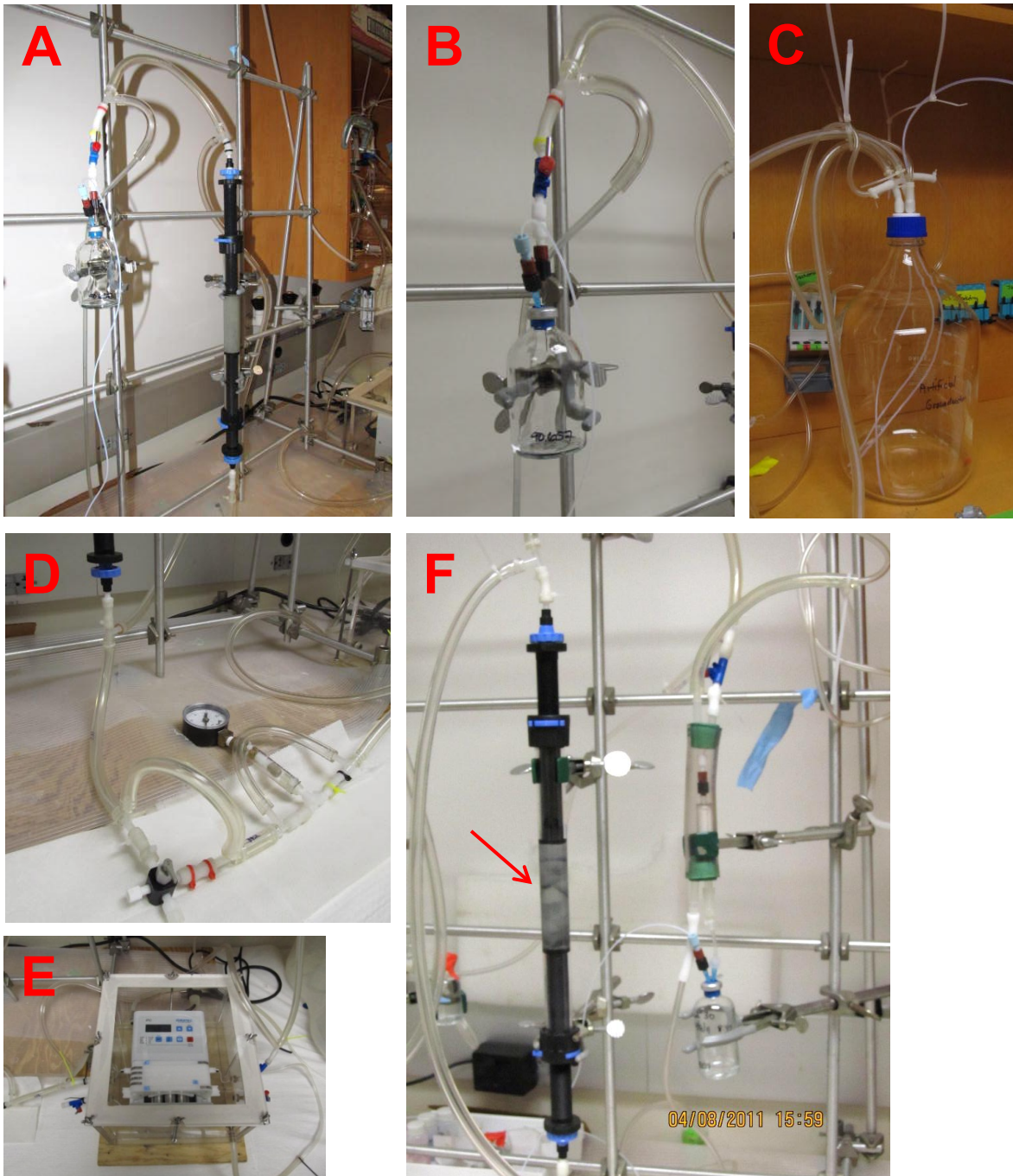
Figure 3.4 Column experimental apparatus illustrating (A) column and effluent collection, (B) effluent tubing with gas purged jacketing to minimize oxygen invasion and effluent collection bottle, (C) influent reservoir with gas mixture purge and outlet lines, (D) influent lines with gas jacketing, (E) peristaltic pump in purged housing. F) Column L2 after 46 days of biostimulation showing dark banding forming in sediment (arrow) and Sterivex filter on outlet for microbial assay test in gas jacketed housing upstream of effluent collection bottle.
