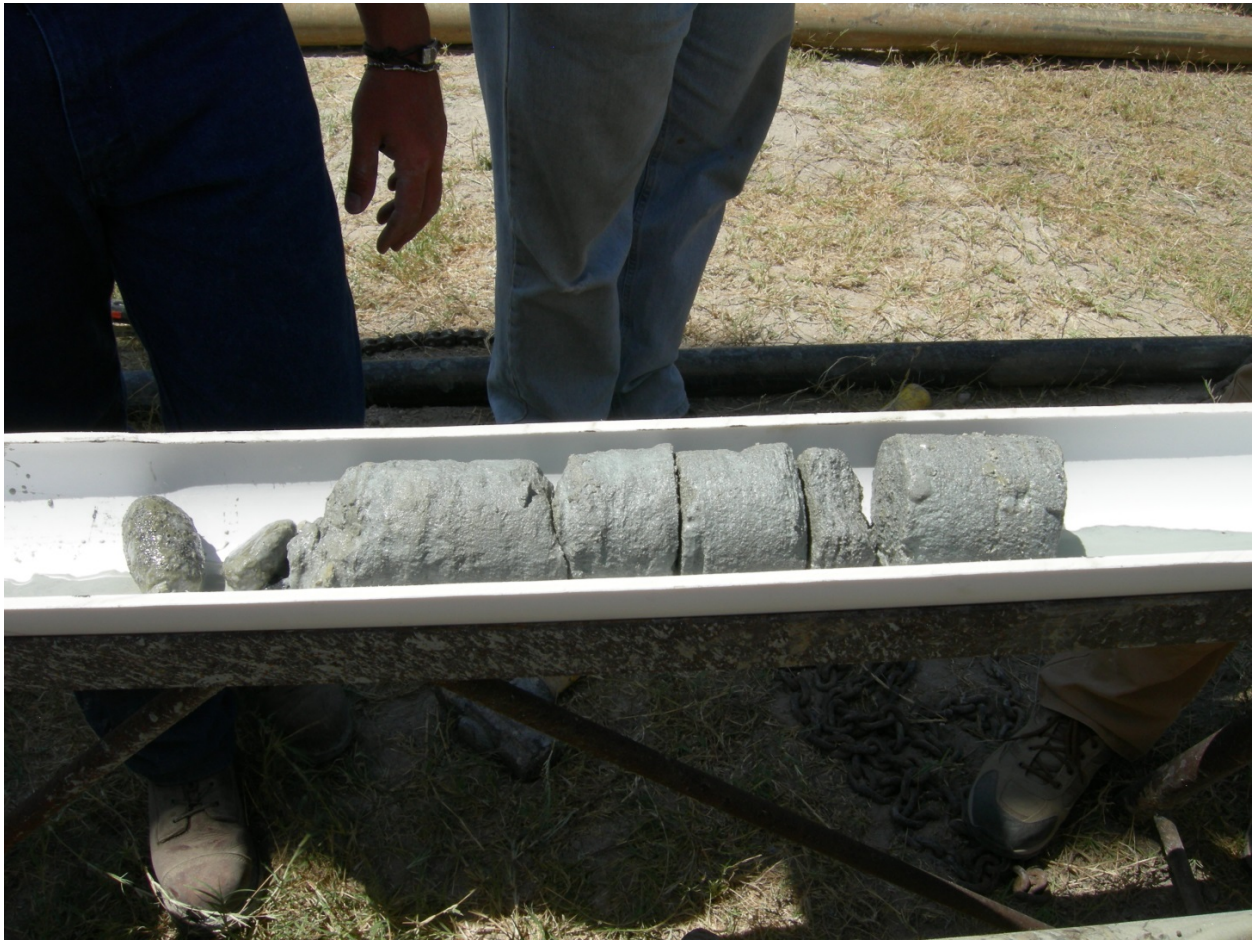
3.3 The sediment sample used for the bioremediation experiments was obtained from a depth of 580-590 feet.
