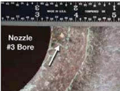
Left photo: Top view of the J-groove weld with an arrow pointing to a crack.
