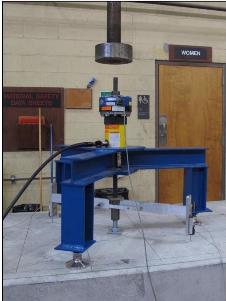
Deep Anchor Test Setup
