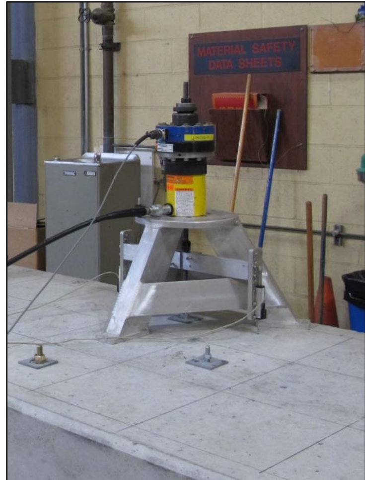
Shallow Anchor Test Setup
