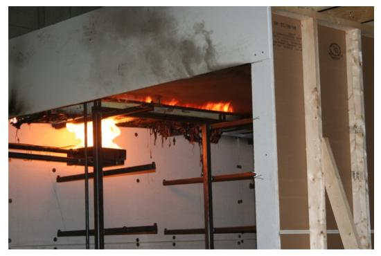
Figure 6-4. Photograph of Test HW-0. Shown are the burner and the lower tray.
