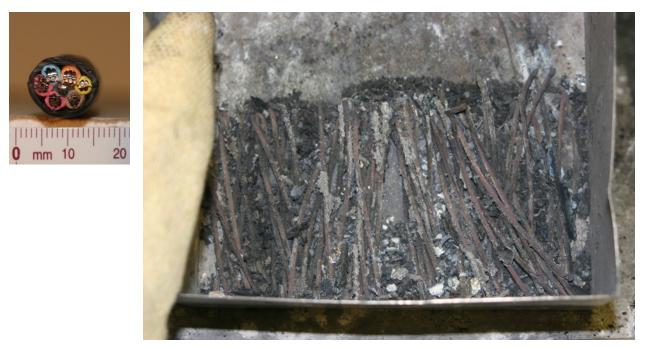
Figure 4-17. Cross section of Cable 806 and photograph of burn residue.
