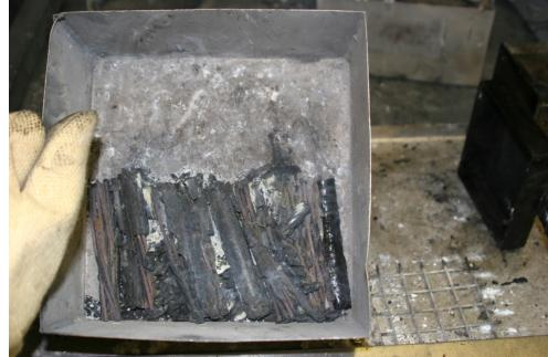
Figure 4-9. Cross section of Cable 802 and photograph of burn residue.
