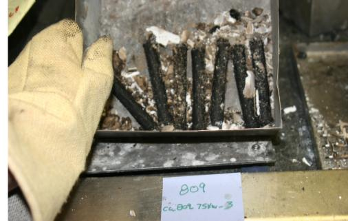
Figure 4-23. Cross section of Cable 809 and photograph of burn residue.
