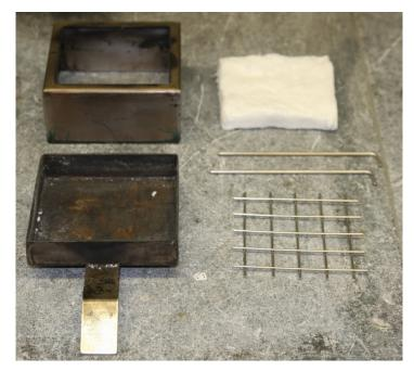
Figure 4-2. Components of the cone calorimeter sample holder.
