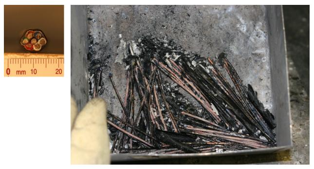
Figure 4-15. Cross section of Cable 805 and photograph of burn residue.
