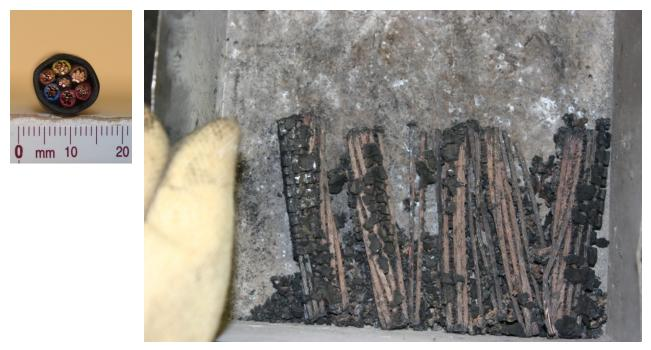
Figure 4-7. Cross section of Cable 801 and photograph of burn residue.
