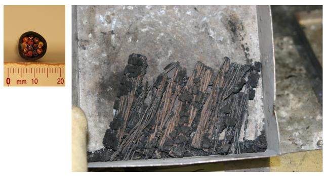
Figure 4-35. Cross section of Cable 815 and photograph of burn residue.
