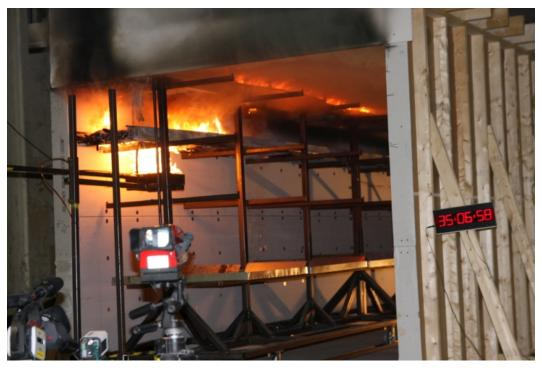
Figure 6-9. Photograph of Test HW-2, from the burner side.
