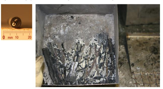
Figure 4-39. Cross section of Cable 817 and photograph of burn residue.
