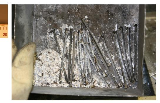
Figure 4-46. Cross section of Cable 822 and photograph of burn residue.
