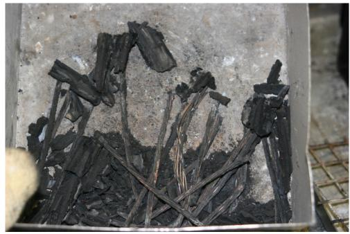
Figure 4-27. Cross section of Cable 811 and photograph of burn residue.
