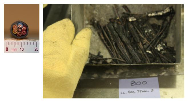
Figure 4-5. Cross section of Cable 800 and photograph of burn residue.
