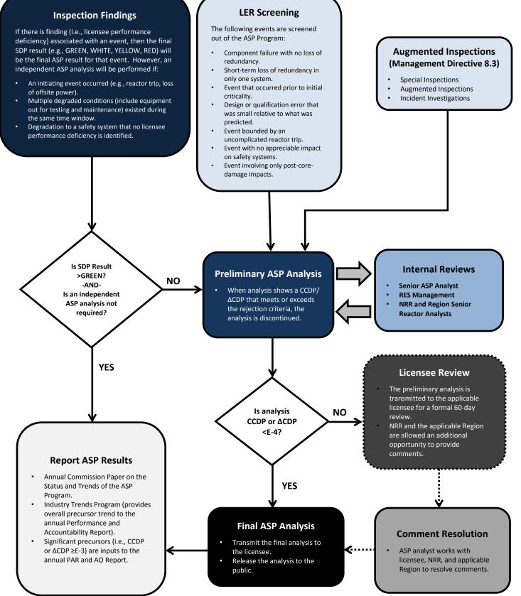
Figure 1. ASP process diagram
