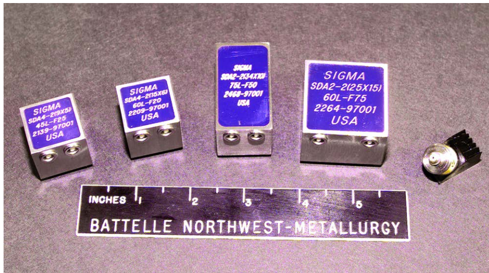
Figure 3-1 Commercial Transducers Typically Used for ISI of Austenitic Materials
