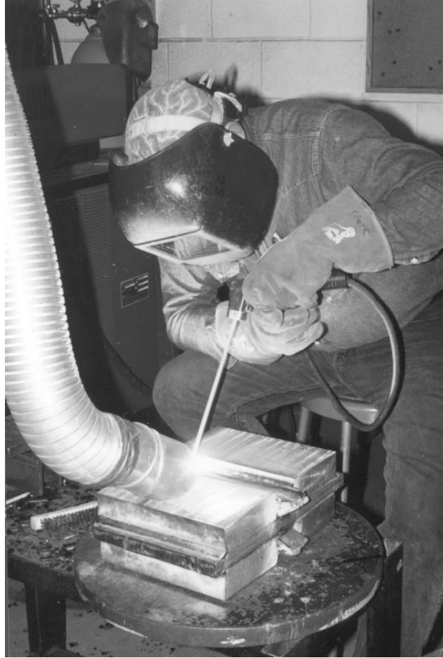
Figure 5-3 Welding of Reactor Internal Mockup Assembly (photo courtesy of FlawTech, Inc., Concord, North Carolina; reprinted with permission)
