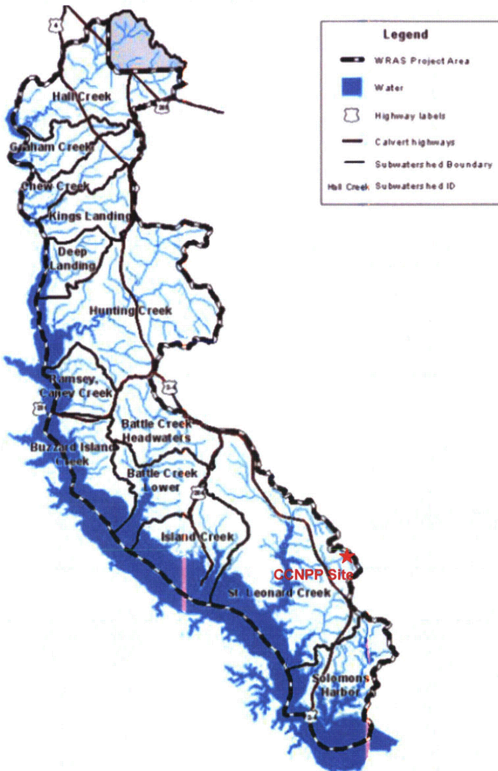
Figure 1.1-6 Sub-Watershed Delineation of the Lower Patuxent River Watershed, which is Indicated as WRAS Project Areas in Legend
