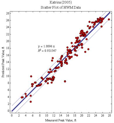
Figure 5: Comparison of observed USACE High Water Marks (HWM) for Hurricane Katrina and the simulation using the H\*WIND/IOKA wind fields. The red points are the values at the recorded USACE HWMs. Thin blue lines display a 1:1 correlation as well as 1.5 ft variance on each side.
