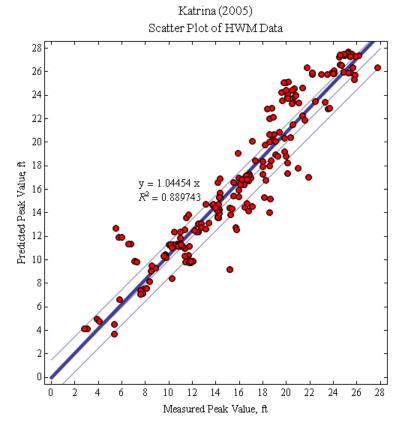
Comparison of observed USACE HWMs for Hurricane Katrina and the simulation using the PBL wind fields. at the recorded USACE HWMs. Thin blue lines display a 1:1 correlation as well as 1.5 ft variance on each side.
