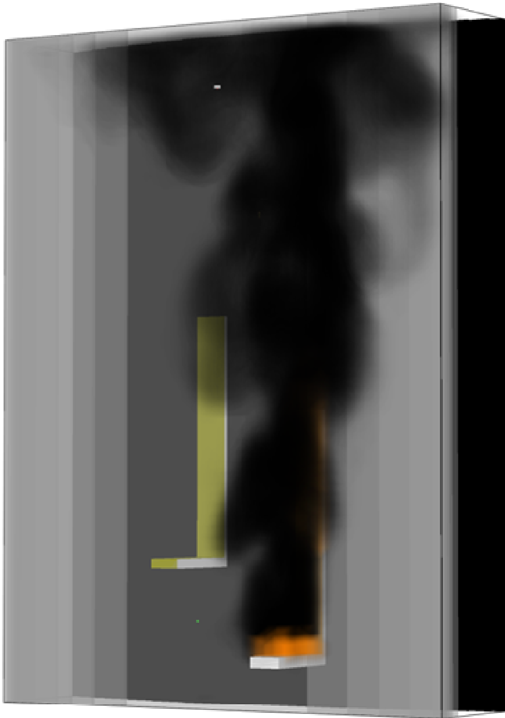
Figure H-4. FDS/Smokeview rendering of the annulus fire scenario.
