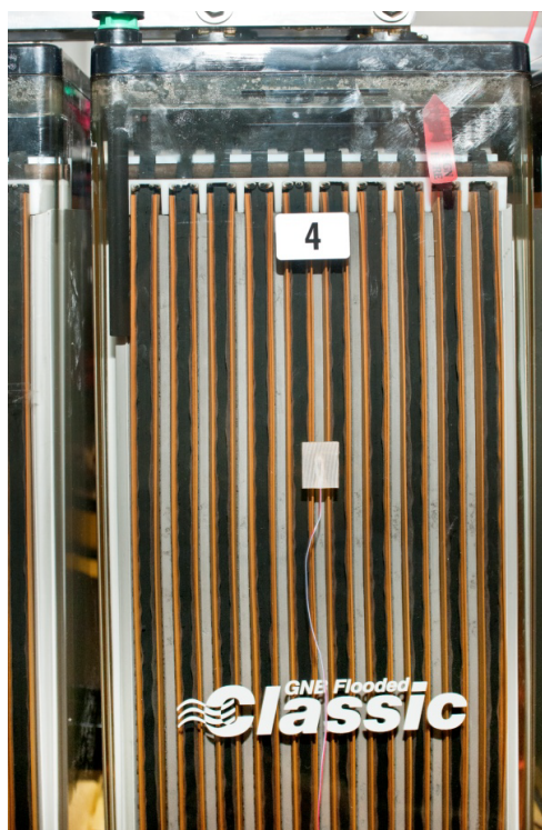
Figure 3-47 Surface Mounted Thermocouple
