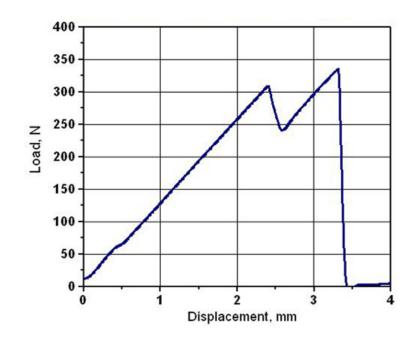
(a) Load-displacement curve for 1<sup>st</sup> 4-mm displacement
