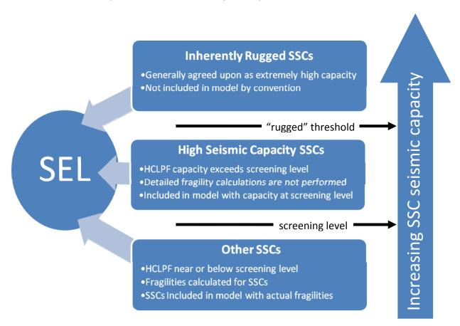
Inherently rugged SSCs are those extremely robust components that are believed to have a seismic capacity beyond any realistic earthquake loading levels (e.g., manual valves). These components are generally mutually agreed upon by the technical community and, by convention, they are not included in SMA or SPRA models. Guidance on inherently rugged components can be found in EPRI NP-6041-SL.
