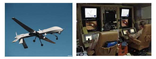
Figure 5-1 Unmanned aircraft system (UAS) - Predator UAV and control station (Aircraft source is http://www.links999.net/robotics/robots/robots\_introduction.html) (Control Station source is http://www.google.com/images)
