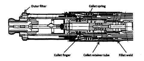
The G003 CTF containing the failed fillet weld was removed from service in 2011. The collet retainer tube axial displacement was observed to be 0.15 inches. The observed displacement is bounded by two dimensions for potential movement of the collet retainer tube:
