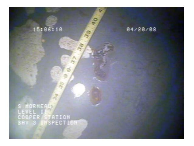
Figure C.1-1 Example of pitting corrosion in torus
