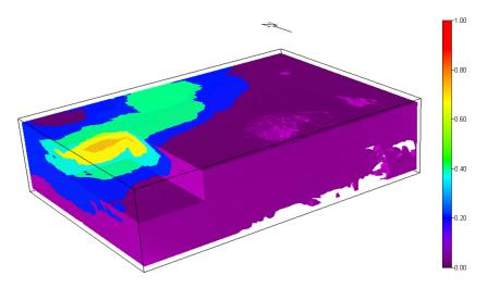
Figure 6.10 Probability of Cs-137 values exceeding 18pCi/g based on geostatistical simulation.
