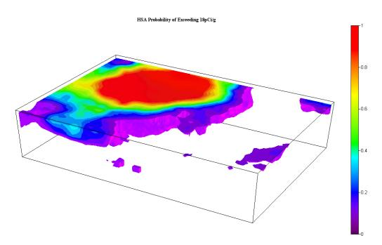
Figure 5.13 Probability of Cs-137 measurements exceeding 18 pCi/g based on HSA data.
