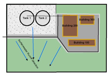
Figure 4.2 Conceptual site model showing facilities, land cover, and surface water runoff direction.
