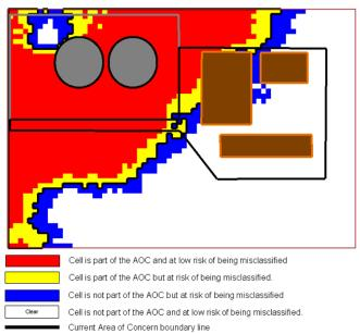
Figure 7.3 AOC map for DCGL of 18+/-5 pCi/g at 2-4 ft.
