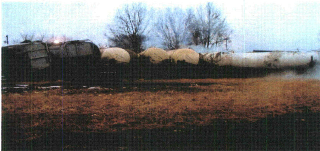
Figure 3-10. Photograph of the Derailment of a Canadian National Freight Train in Tamaroa, Illinois, on February 9, 2003. This Photograph Shows a Portion of the Railcar Heap Resulting From This Accident. The Arrangement of Railcars Illustrates the Concept of an Accordion Arrangement of Derailed Railcars. This Image Is From National Transportation Safety Board RAR-05/01.
