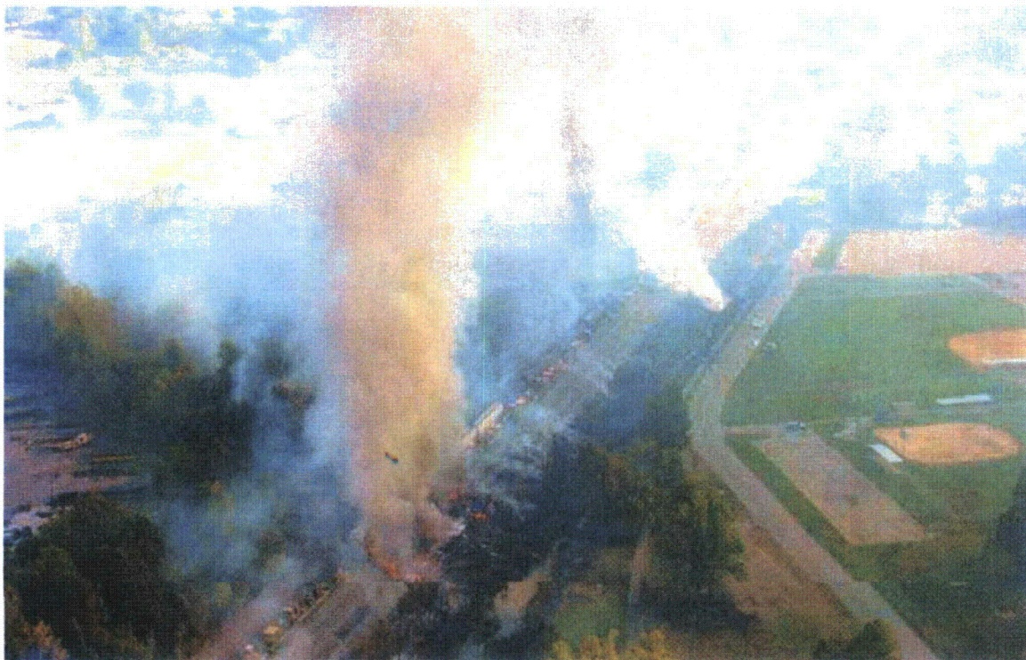
Figure 3-13. Aerial Photograph of the Train Derailment and Fire in Texarkana, Arkansas, on October 15, 2005. The Widespread Fire Was the Result of Flowing Flammable Gas, Which Filled a Large Area Before Igniting in an Occupied House Along the Rail Line. This Image Is From National Transportation Safety Board RAB-06/04.
