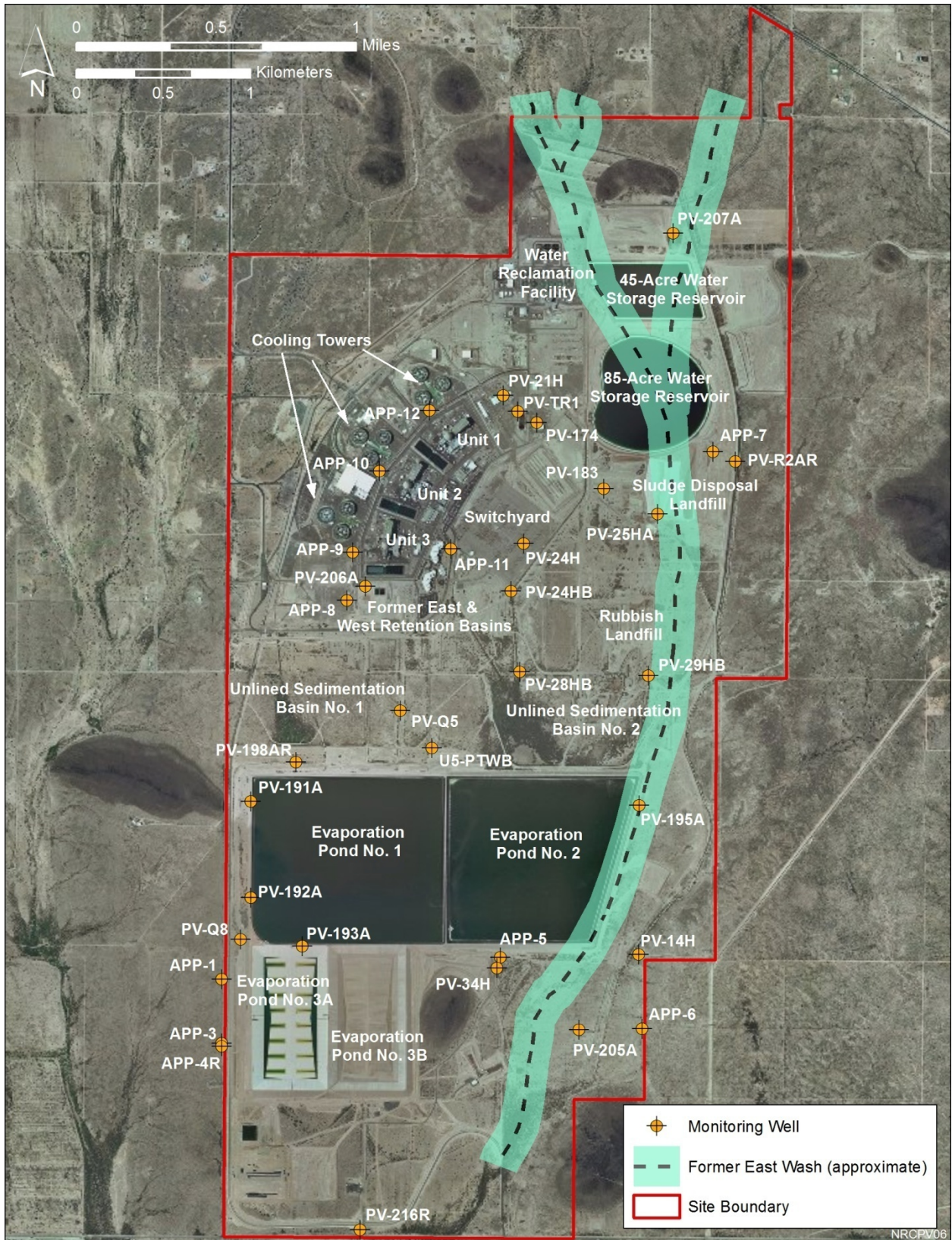
Figure 2.1.7-1 PVNGS Surface Impoundments, Landfills, and Monitoring Wells
