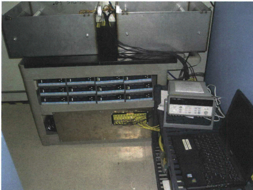
Figure 6 PID Controllers Used to Set and Control the Temperature of the Cartridge Heaters
