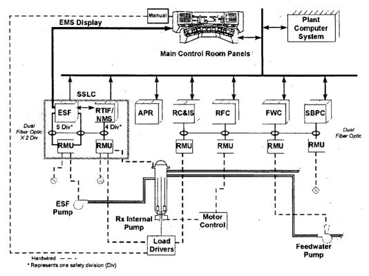
Fig. 4.10. Overall architecture of Lungmen 1&C systems. (Adapted from Ref. 108.)
