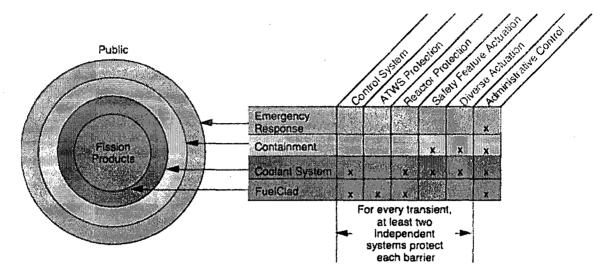
Fig. 2.2. Representation of I&C system architecture lines of defense. (Source: Gary Johnson, IAEA. Used with permission)
