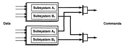
Fig. 4.3. Functionally diverse subsystems.
