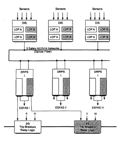
Fig. 4.9. Digital safety system at Dukovany Nuclear Power. (Adapted from Ref. 107.)
