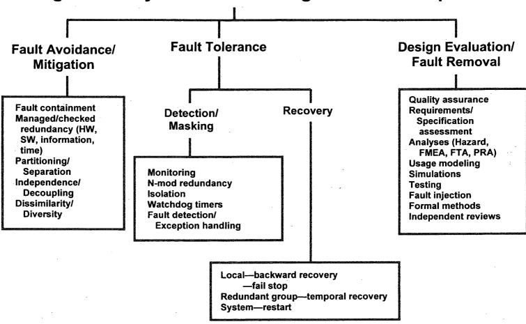
Fig. 2.1. Fault management techniques for digital I&C systems.
