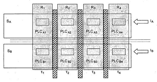
Fig. 5.1. ISTec diversity usage approach for a parallel diverse redundant architecture. (Adapted from Ref. 18.)
