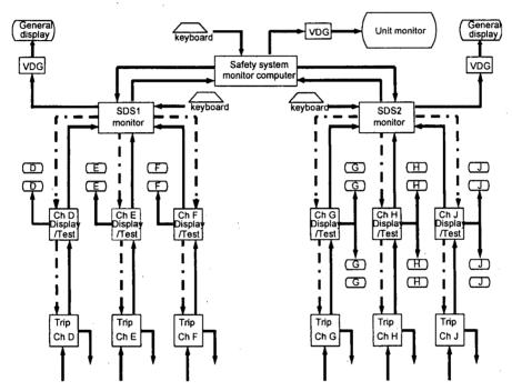
Fig. 4.4. Fully computerized shutdown system.
