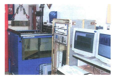
Figure 2.5 SAFT-UT Immersion Inspection of Small Weld Segments
