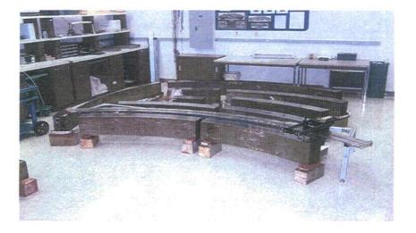
Figure 2.3 Large Weld Segments from the Shoreham Vessel
