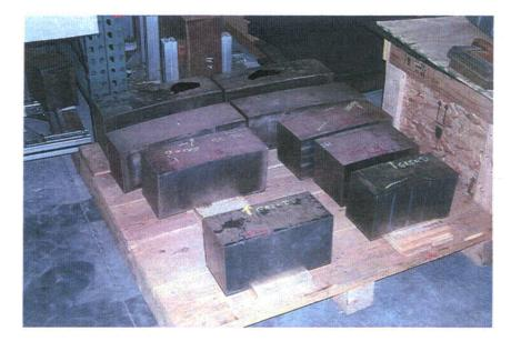
Figure 2.4 Photo of Small Weld Segments from Hope Creek Unit 2 and River Bend Unit 2 Vessels for Immersion Testing
