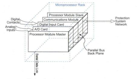
Fig. 2.1. Generic microprocessor-based rack.
