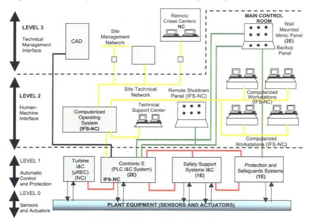
Fig. 3.1. I&C architecture of Chooz B (N4) Plant.
