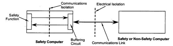
Fig. 4.1. Concept of communication buffering from IEEE 7-4.3.2-2003 Annex E.
