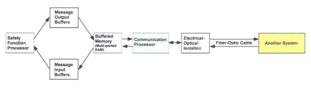
Fig. 4.2. Possible implementation of communication buffering using multiported memory.
