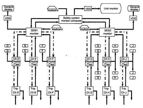
Fig. 3.4. Reactor protection system architecture.
