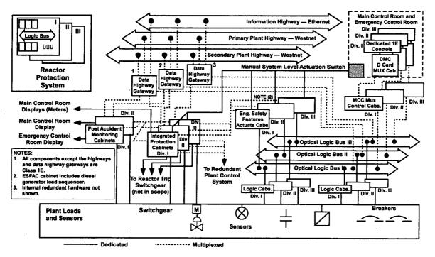
A function-level diagram of the protection system is given in Fig. 3.7.
