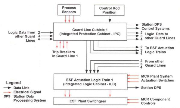
**Fig. 3.2.** Sizewell B protection system diagram illustrating communications within a division. *Adapted from* G. B. Moutrey and G. Remley, "Sizewell B power station primary protection system design application overview: Electrical and Control Aspects of the Sizewell B PWR," International Conference on 14–15 September 1992, p. 221–231.
