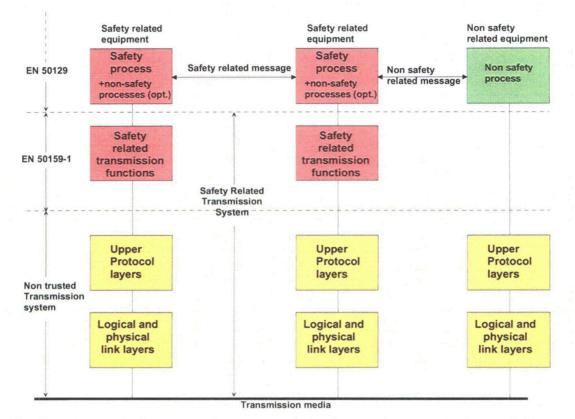
**Fig. G.4. Communication model using nontrusted closed transmission system.** *Source*: J. Alanen et al., *Safety of Digital Communications in Machines*, VTT Research Notes 2265, October 2004. Permission to use this copyrighted material is granted by J. Alanen.
