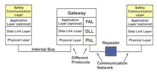
**Fig. 4.4.** Three-level layer model with SCL applied to a safety system network. This figure is similar to Fig. 2.3 except with the SCL added.
