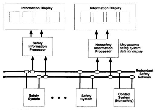
Fig. 1.2. Simplified generic I&C architecture for sending safety system information to multidivisional display stations.
