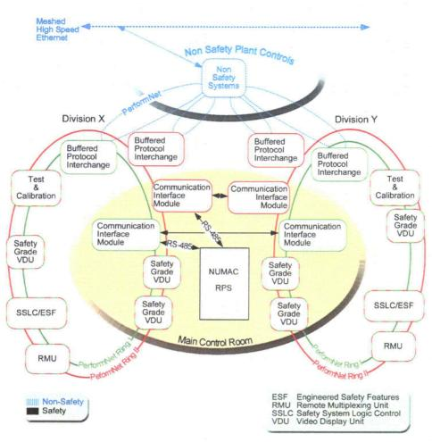
Fig. 3.6. Lungmen essential multiplexing system network topology.
