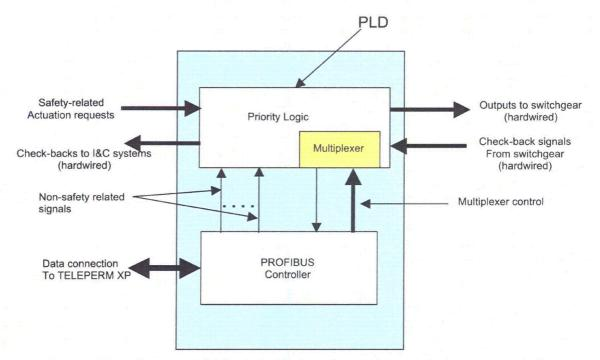
Fig. 3.9. Block diagram of Olkiluoto 3 priority and actuation module (based on Ref. 32).
