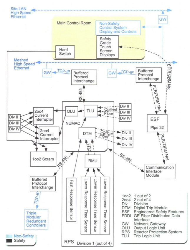
Fig. 3.5. Lungmen reactor protection system communications paths and protocols.
