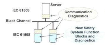
Fig. 4.5. Illustration of black channel implementation.
