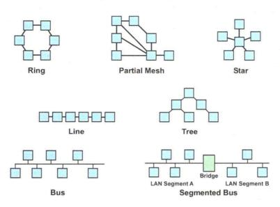
Fig. 2.4. Typical communications network topologies.
