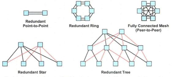
Fig. 2.6. Communication networks with redundant topological features applicable to safety.
