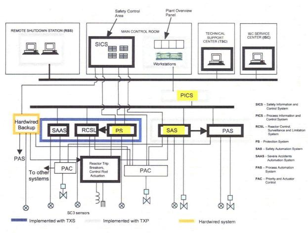
Fig. 3.8. Olkiluoto 3 I&C architecture. Adapted from J. Hyvarinen, STUK (see Ref. 32).
