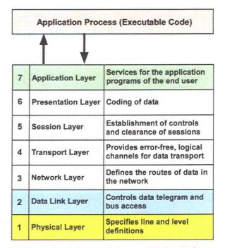
Fig. 2.3. OSI model layers and their relation to executable code.
