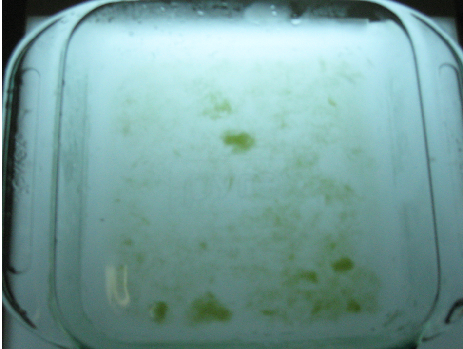
Figure 3. Fiber slurry appearance after debris preparation
