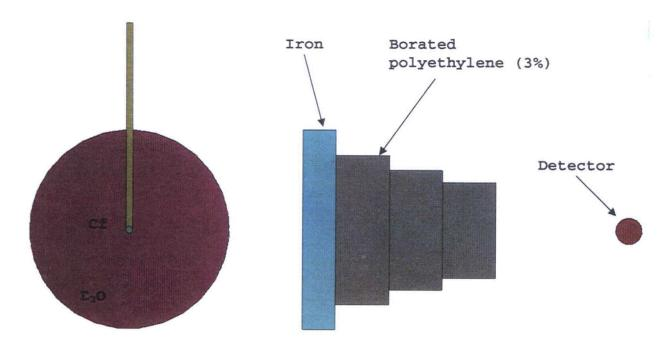
Fig. 3.48 Monaco model of <sup>252</sup>Cf source in heavy water experiment.
