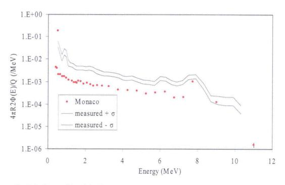
Fig. 3.46 Comparison of the photon calculation to the measurement of the 70 cm shield.
