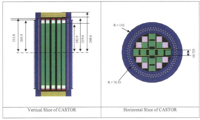
Fig. 3.1 Views of cask for storage and transport of radioactive material (CASTOR). (Dimensions in centimeters.)
