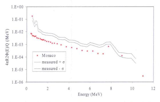
Fig. 3.44 Comparison of the photon calculation to the measurement of the 50 cm shield.
