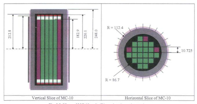
Fig. 3.2 Views of MC-10 cask. (Dimensions in centimeters.)
