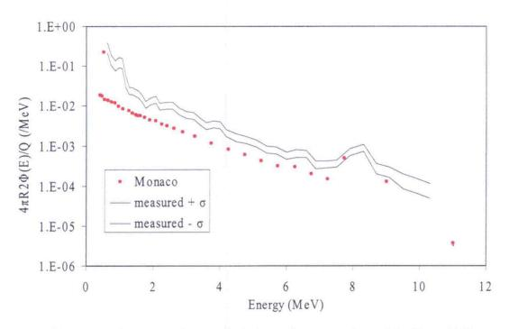
Fig. 3.43 Comparison of the photon calculation to the measurement of the 40 cm shield.
