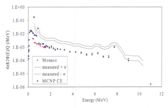
Fig. 3.47 Photon flux through the 70 cm shield as calculated by Monaco and MCNP5.
