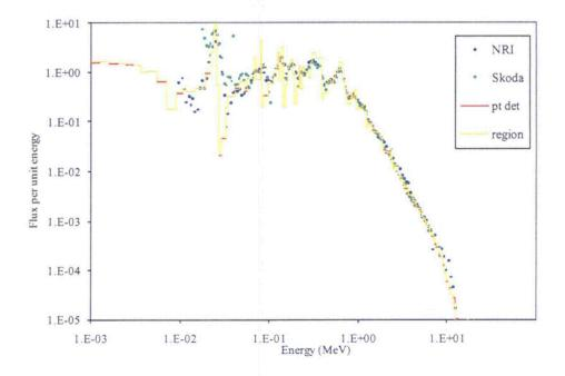
Fig. 3.53 Monaco output (ENDF/B-VI.8 fine-group library) for total flux at 10 cm using two different tallies compared to the two sets of measured data.
