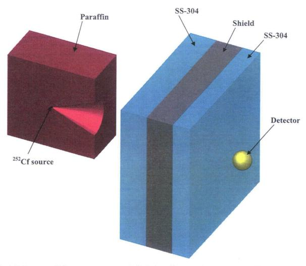
Fig. 3.57 Neutron shielding experiment example (half of paraffin removed to show source inside cone).
