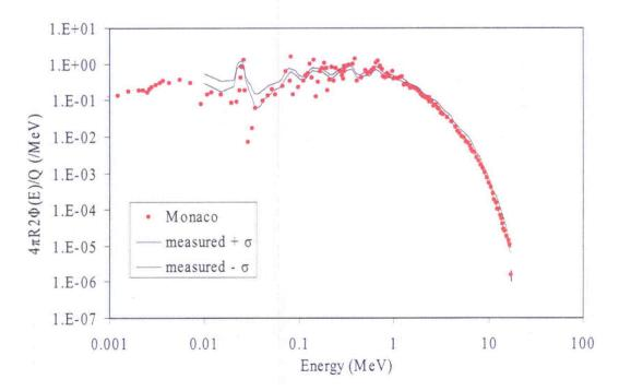
Fig. 3.36 Comparison of the neutron calculation to the measurement of the 20 cm shield.
