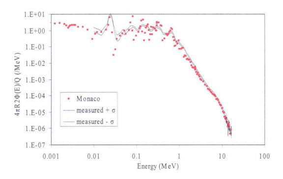
Fig. 3.41 Comparison of the neutron calculation to the measurement of the 70 cm shield.
