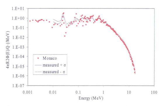
Fig. 3.37 Comparison of the neutron calculation to the measurement of the 30 cm shield.
