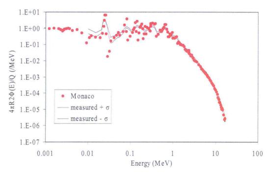
Fig. 3.38 Comparison of the neutron calculation to the measurement of the 40 cm shield.
