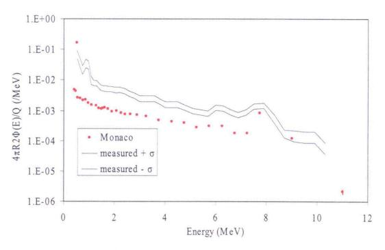
Fig. 3.45 Comparison of the photon calculation to the measurement of the 60 cm shield.
