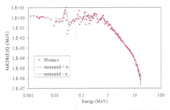
Fig. 3.39 Comparison of the neutron calculation to the measurement of the 50 cm shield.
