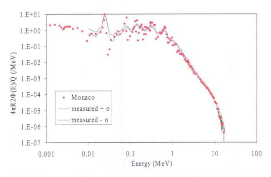
Fig. 3.40 Comparison of the neutron calculation to the measurement of the 60 cm shield.
