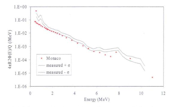
Fig. 3.42 Comparison of the photon calculation to the measurement of the 30 cm shield.
