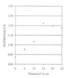
Fig. 3.59 Type 2a results—25 cm of stainless steel first, then polyethylene.
