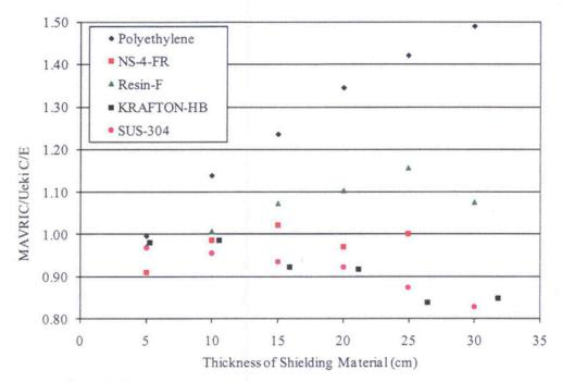
Fig. 3.58 Ratio of MAVRIC calculation of neutron detector dose rate to experimental measurement.
