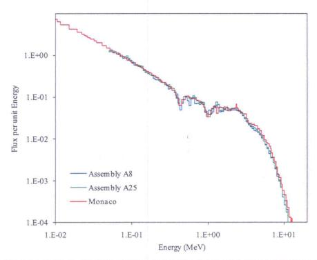
Fig. 3.49 Comparison of the Monaco (ENDF/B-VI.8) results and the measured data.
