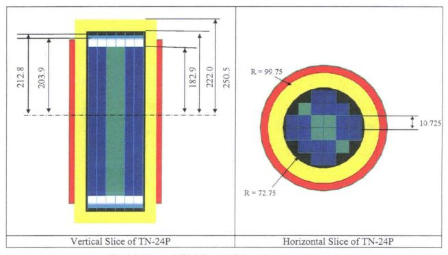
Fig. 3.3 Views of TN-24P cask. (Dimensions in centimeters.)
