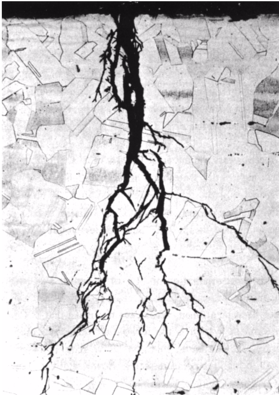
Figure 2.3.4-58. Typical Example of Transgranular Stress Corrosion Crack in Stainless Steel
