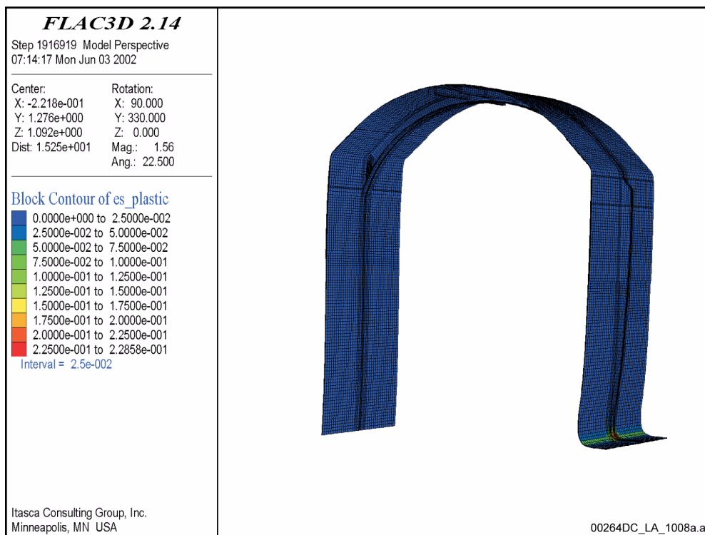
Figure 2.3.4-82. Deformed Shape and Contours of Plastic Shear Strain in the Failure State for the Drip Shield (top) Components Not Thinned, and, (bottom) Components Thinned 10 mm
