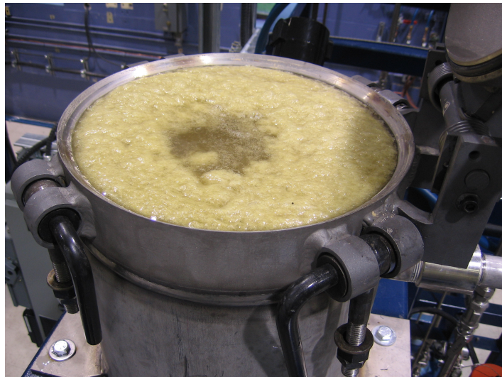
Figure 3: Debris Slurry Poured Into Debris Addition Tank
