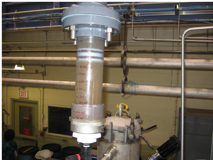
Figure 8: Injection of Chemicals into a Multi-Loop Rig Test Loop
